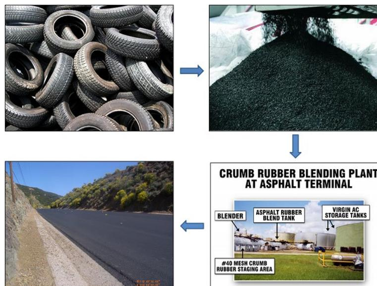
Figure 28. Rubberized Asphalt Concrete using Crumb Rubber
