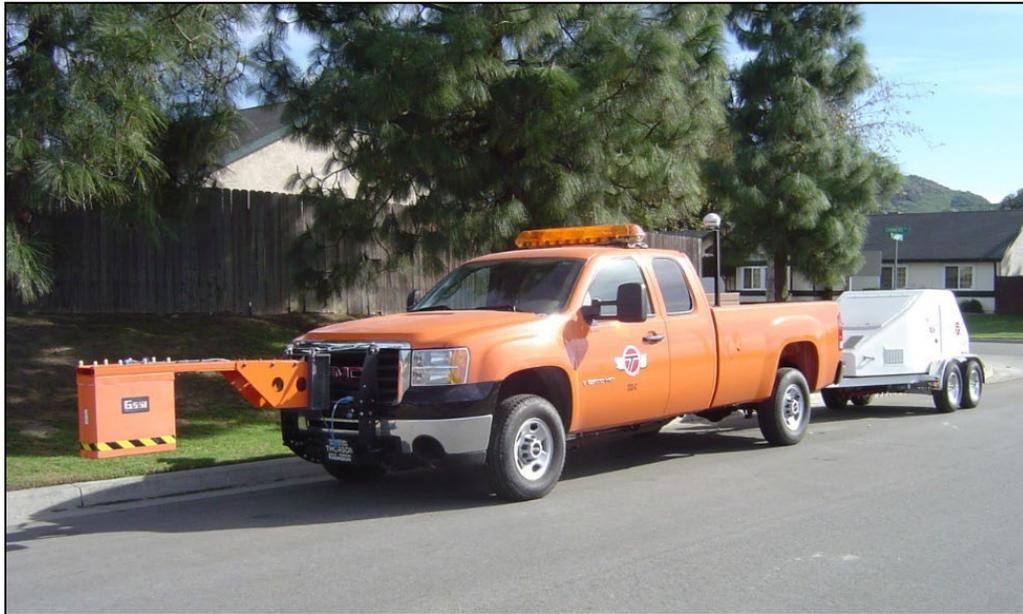
**Figure 9. FWD and GPR Data Collection Equipment**
