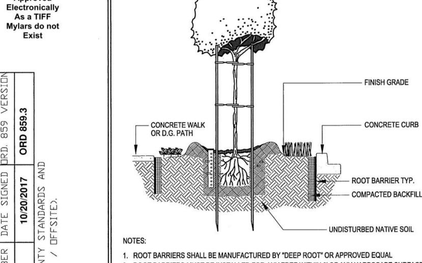
2. ROOT BARRIERS MUST BE INSTALLED FOR ANY TREE WITHIN 8' OF ANY HARDSCAPE SURFACE OR DECOMPOSED GRANITE PATH
