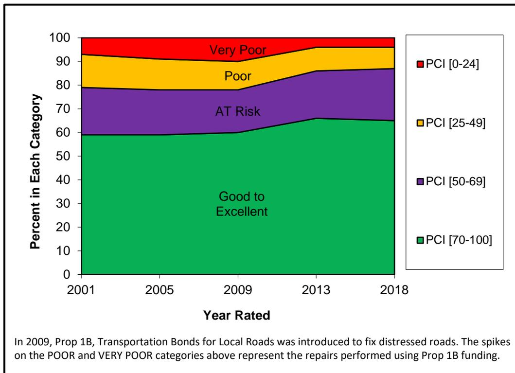
**Figure 3. Pavement Condition Trendline (Countywide)**
