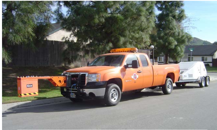
Figure 15. FWD and GPR Data Collection Equipment
