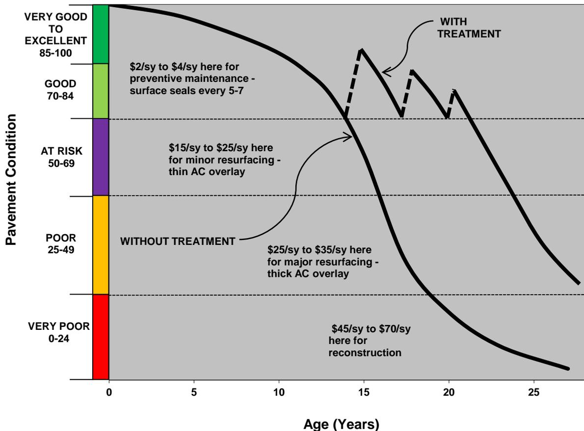
Figure 10. Pavement Deterioration Curve With and Without Treatment
