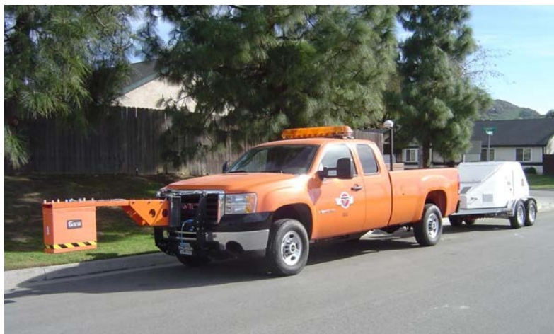
Figure 18. FWD and GPR Data Collection Equipment
