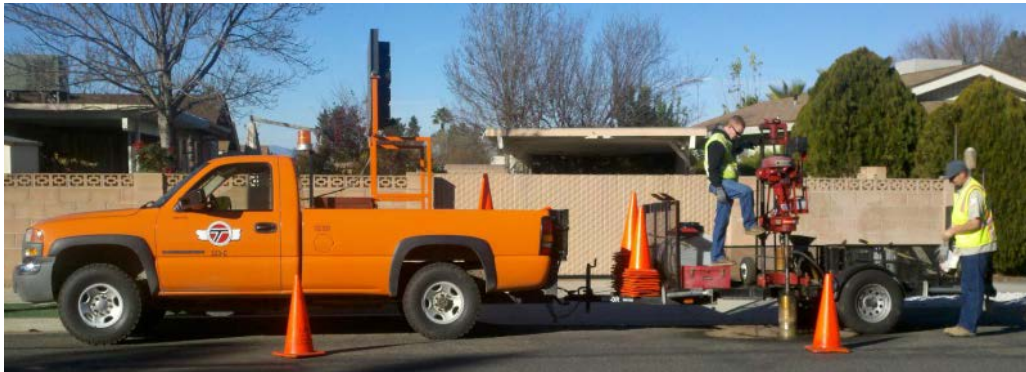
Figure 17. County's Coring Rig
