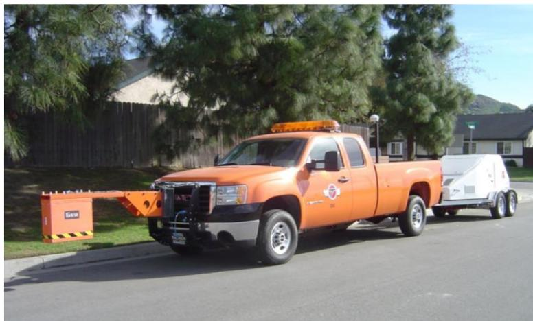
**Figure 17. FWD and GPR Data Collection Equipment**
