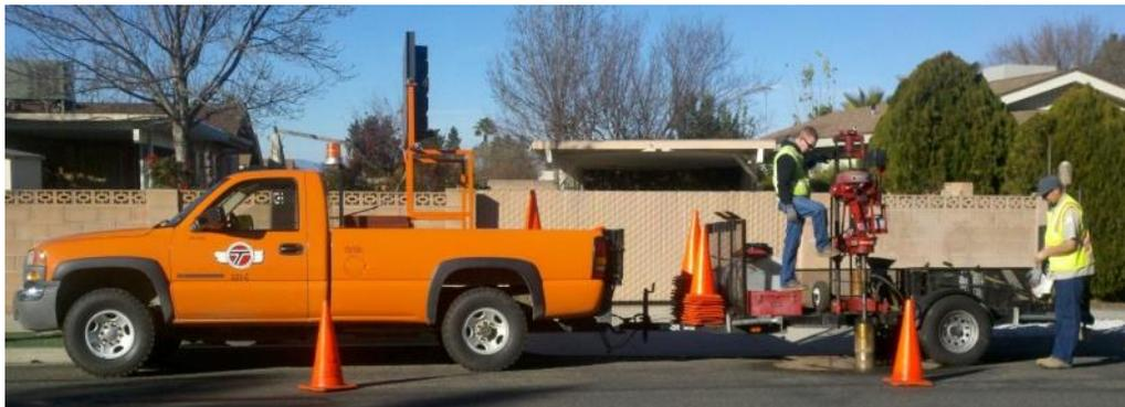
**Figure 16. County's Coring Rig**
