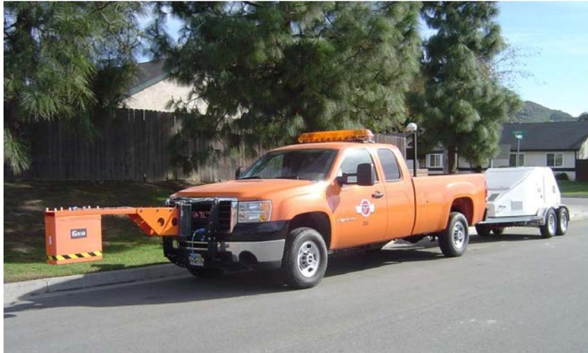
**Figure 15. FWD and GPR Data Collection Equipment**
