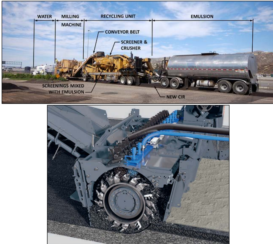
Figure 27. Cold In-Place Recycling (CIR)
