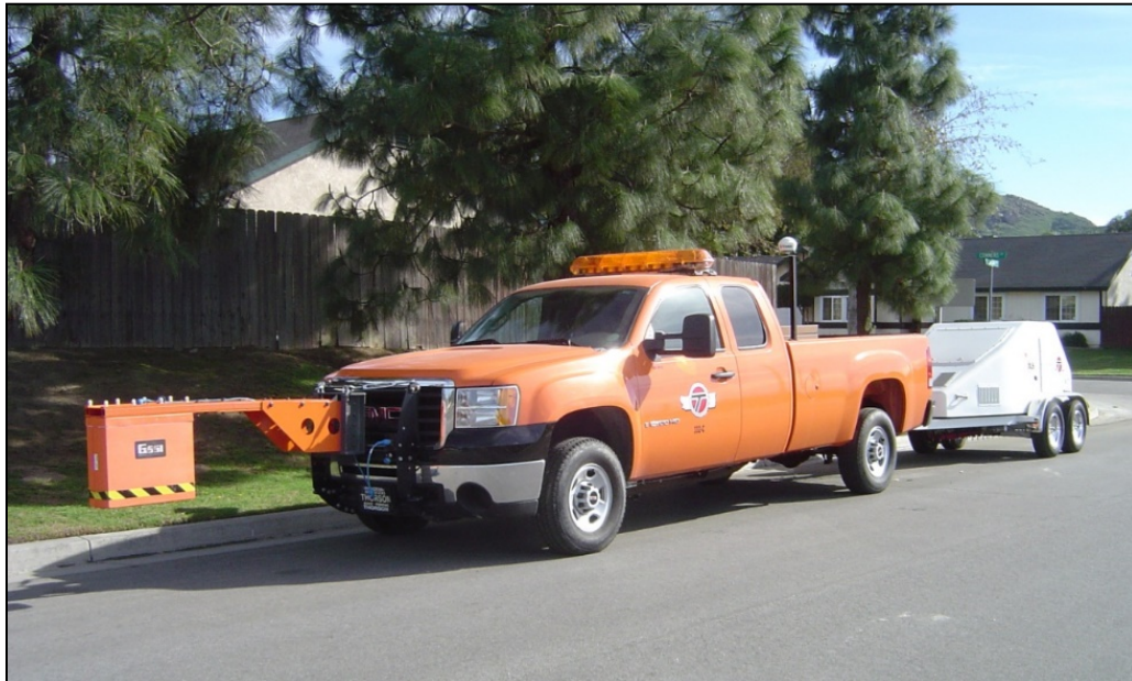
Figure 9. FWD and GPR Data Collection Equipment
