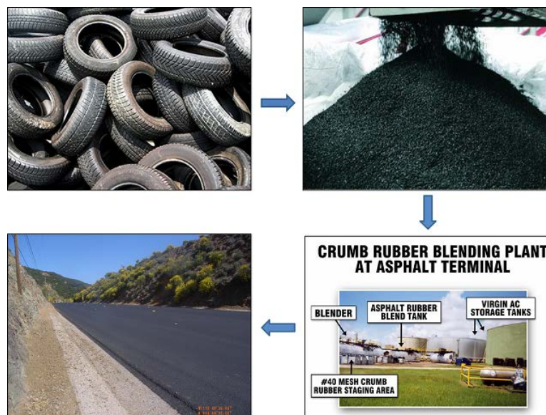
Figure 28. Rubberized Asphalt Concrete using Crumb Rubber
